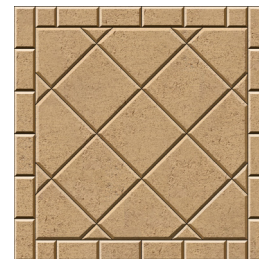
45° Stack Bond / Diamond with flat header course
