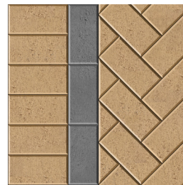
45° Herringbone with contrasting stretcher inlay and header
